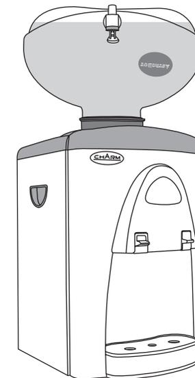
2. Take off the cover sticker from the smart cap. Turn the tank upside down and hook up with any counter top drink water systems / coolers.
